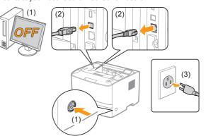
When installing or removing the optional accessories, be sure to turn the printer OFF, unplug the power plug, and then disconnect all the interface cables and power cord from the printer. Otherwise, the power cord or interface cables may be damaged, resulting in a fire or electrical shock.
